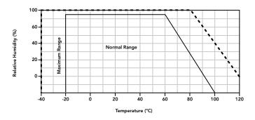
Long term exposure (more than 60 hours) to conditions outside the normal range, shown above, may result in a temporary drift of up to +3% RH. Once within the normal range again it will return to the calibrated state.
