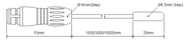
Typical Applications Composting Cable lengths 1.5, 3 & 10m
