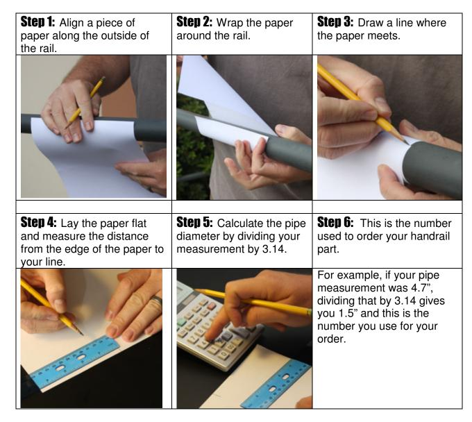
Instead of paper, you can also wrap a string around your hand rail, mark the point at which the string overlaps and measure the length of the string.
