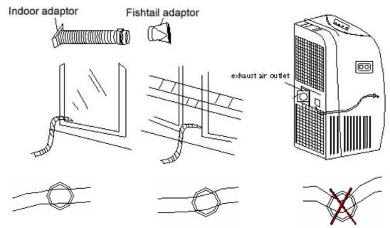
Avoid kinks and bends in the exhaust hose as this will cause expelled moist air to build up causing the unit to overheat and shut down.
