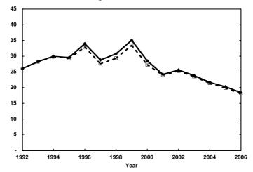
**Figure 1.** Energy return on investment for oil and gas production worldwide. Quality-corrected (solid line) and heat equivalent (dashed line) estimates are shown.
