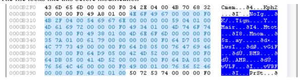
Knocks are stored in the symbol KnkDetAdap.KnkCntCyl (in my file is the address of F01A36) is 8 bytes long (2 bytes per cylinder) and it's updated every time knock is detected. The value of the first cylinder has address F01A36, second cylinder (increase 2 bytes) is then F01A38, F01A3A third and fourth on F01A3C.
