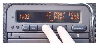
A list will appear that you can scroll through with the +/- buttons. There is a summary on what the acronyms stand for here. Press the SET button once to freeze a value and keep it so that when you scroll only the lower value is replaced.
