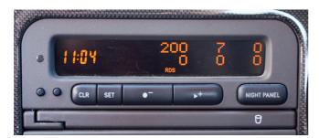
Press and hold either + or - button to see which parameter is in each cell..
