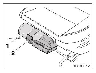
The fixing stud on the fire extinguisher bracket must be inserted in the outlet aperture of the fire extinguisher.
