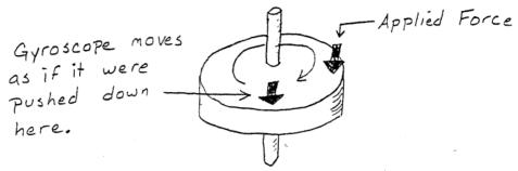
The gyroscope principle says that an applied force will act a quarter rotation later. If a gyroscope is rotating counterclockwise and a force is applied to the left side of its frame, then the gyroscope will tilt as if the force were applied to the near side of its frame. See the diagram below.
