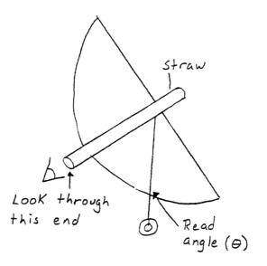
To use, view through the straw so that you are looking at the object that you want to measure. Read the angle from where the thread crosses the protractor.
