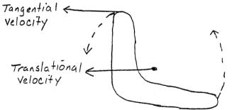
The arm on top has a greater velocity relative to the bottom arm. Therefore, the lift on the top arm is greater than the lift on the bottom arm. The net lift is on the top arm. Due to the gyroscopic principle, the net lift acts in front of the boomerang. This is what causes the boomerang to turn. Added to it, the directional lift of the boomerang is off to the side, which
