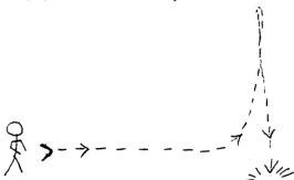
As a boomerang travels in a circle, it flattens out horizontally. There are three ways to account for this. Though all three explanations are described, the preferred description used in class follows.
