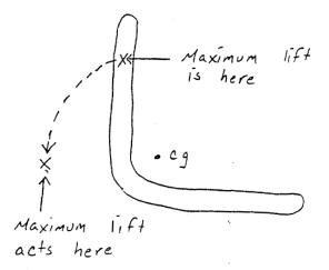
To show the effect of the rotation, throw a plastic boomerang horizontally (side-armed throw). The net lift this time is on the right side of the boomerang. The gyroscopic principle makes the force act at the front of the boomerang. Also, the directional lift is upward. Below is the path that the boomerang will travel. This is why all boomerangs are thrown vertically (or near vertical), but never horizontally (side-armed throw).
