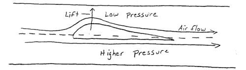
The same forces act on boomerangs and gliders that have cambered wings. Even though the airfoils are thin, the airflow on the top of the wing is greater than the bottom of the wing. The difference is still enough to generate lift.
