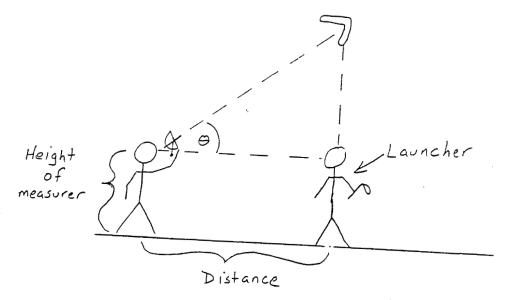
Another method to find the height, which is also helpful if the object is drifting away from the thrower is to use a non-right angle method. Two people are needed to measure the angles simultaneously and one must be behind the other. The distance between the two angle measurers must be known. Use the following formula:
