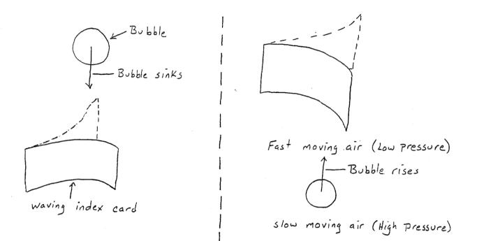
Waving the card causes the air to move faster and creates a lower pressure area. The bubble will move towards the lower pressure area. On a wing, the shape of the wing causes a lower pressure area on the top of the wing, causing the wing to rise (Lift).
