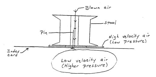
The air coming out of the spool's bottom between the card and the spool is moving very fast. Therefore, it has a low pressure when compared to the air on the other side of the card. The air on the other side of the card is not moving at all. Therefore, the pressure underneath the card is greater than the pressure on the top of the card. This greater pressure is lifting the card up against the spool.
