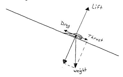
Gliders are able to stay aloft for extended periods of time by using updrafts of air from wind hitting an incline or thermals. The analogy I use for my students to understand this is flying a glider inside of a GIANT elevator being lifted by a crane. If you are inside of a stationary elevator, flying your glider, the glider descends as it normally would.
