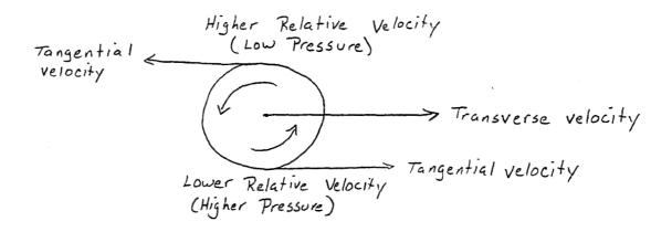
At the top of the cups, the spin along with the forward movement of the cups, creates an even higher air velocity at the top of cups than the velocity at the bottom of the cups. The greater velocity means a lower pressure. Therefore, the pressure on the bottom of the cups is greater than the pressure on the top of the cups. This is part of the reason why the cups rise when launched.
