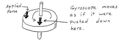
Another concept relating to the gyroscopic principle is gyroscopic precession. Using the same gyro and a piece of string, lay the gyro so that its disk is now rotating along a vertical axis. Loop the piece of string and place one of the posts of the gyro through the loop. The gyro, will remain horizontal, but will also rotate around the piece of string. This is much more dramatic and easier to see if you replace the gyro with a bike wheel with two posts as handles in the center of the wheel.
