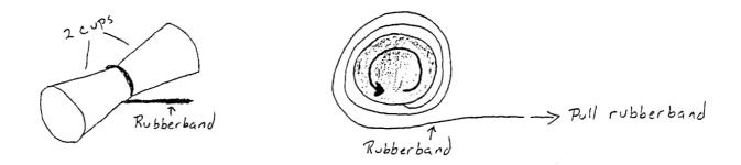
When the cups leave the rubberband it will be rotating with a back-spin. There will be a tangential component of velocity to the edge of the cups. The cups will also have a transverse velocity. Recall that the velocities associated with lift are velocities relative to the surface. Look at the diagram below.
