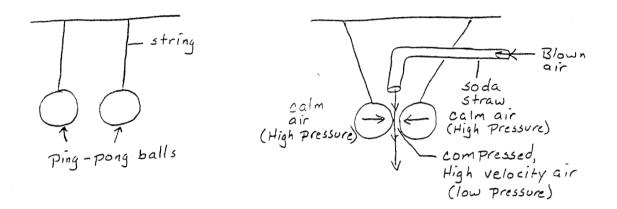
The air between the balls is moving faster than the air on the outside of the balls. Therefore, as demonstrated above, the pressure between the balls is less than the pressure on the outside of the balls. The greater pressure on the outside pushes the ping-pong balls together.
