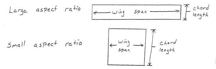
There is a limit to the aspect ratio. If the wings become too long, then the material of the wings may flex too much and possibly fail. For example, a short piece of paper held out horizontally will have nearly no flex and will be fairly rigid. The longer the piece of paper becomes, the more flexing in the paper will occur.
