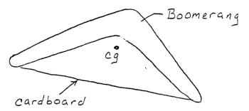
Toss the boomerang vertically up in the air with a spin on it. Don't use too much spin or the boomerang may curve to the side. Notice that the boomerang rotates around the cg that was marked in the experiment.
