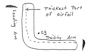
The dotted line along the boomerang shows where the thickness of the boomerang is the greatest. On each end is a cross-section of the wing tips.
