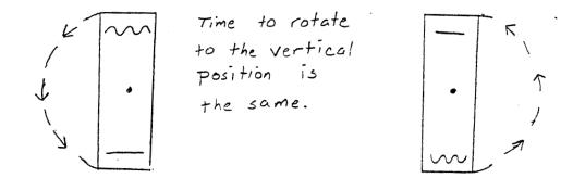
But a boomerang is curved. One arm will reach the vertical position quicker than the other. This may not seem obvious at first. Take a boomerang and lay it on a table like below on the left. Then rotate the boomerang so that the other arm is now vertical
