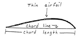
Cambering is the process of making a thin airfoil. This is easily done with your fingers. Below is a diagram of approximately how much of the whole wing must be cambered based on the wing's chord length. Depending on the type of flight performance needed, different variations of cambering are needed.
