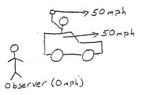
The student in the car throws the ball in front of him at 30mph. The speed of the ball relative to student in the car is 30mph. The speed of the ball relative to the observer alongside of the road is 80mph (50mph + 30mph).
