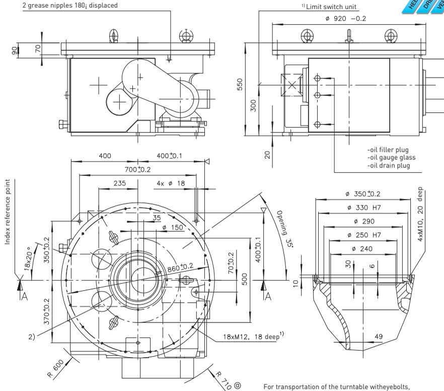
For transportation of the turntable with eyebolts, 3 tapped holes M24x40 deep have been arranged on  $\varnothing 580$ .
