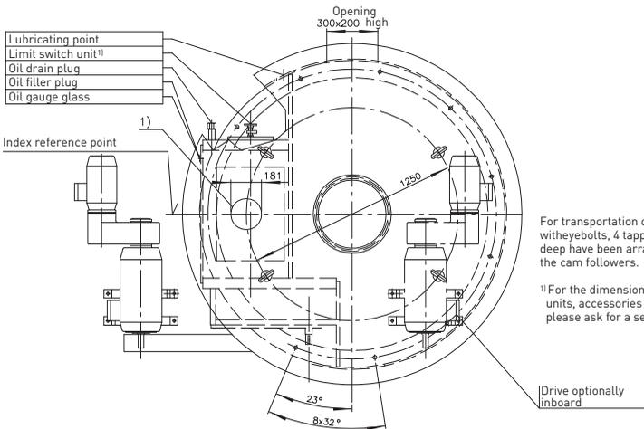
For transportation of the turntable with eyebolts, 4 tapped holes M30x45 deep have been arranged in the area of the cam followers.
