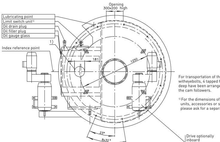
For transportation of the turntable with eyebolts, 4 tapped holes M30x45 deep have been arranged in the area of the cam followers.
