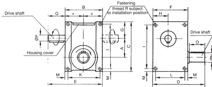
Shaft end according to DIN 748, fluted according to DIN 6885 page 1, P 9
