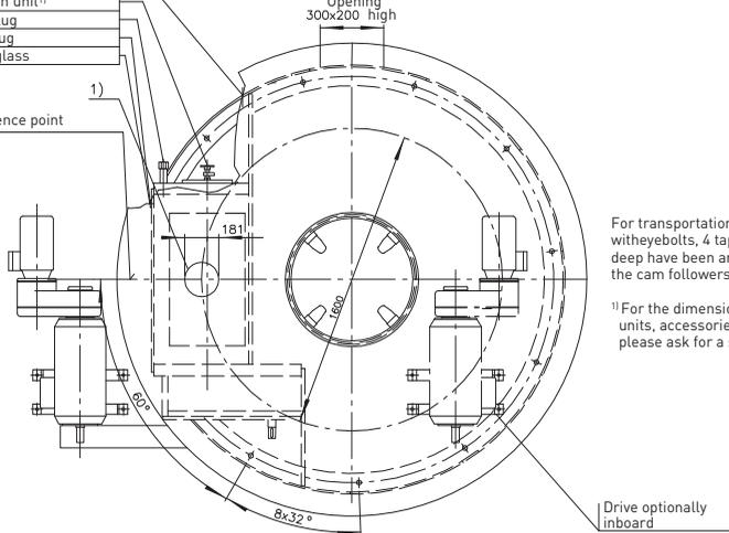
For transportation of the turntable with eyebolts, 4 tapped holes M30x45 deep have been arranged in the area of the cam followers.
