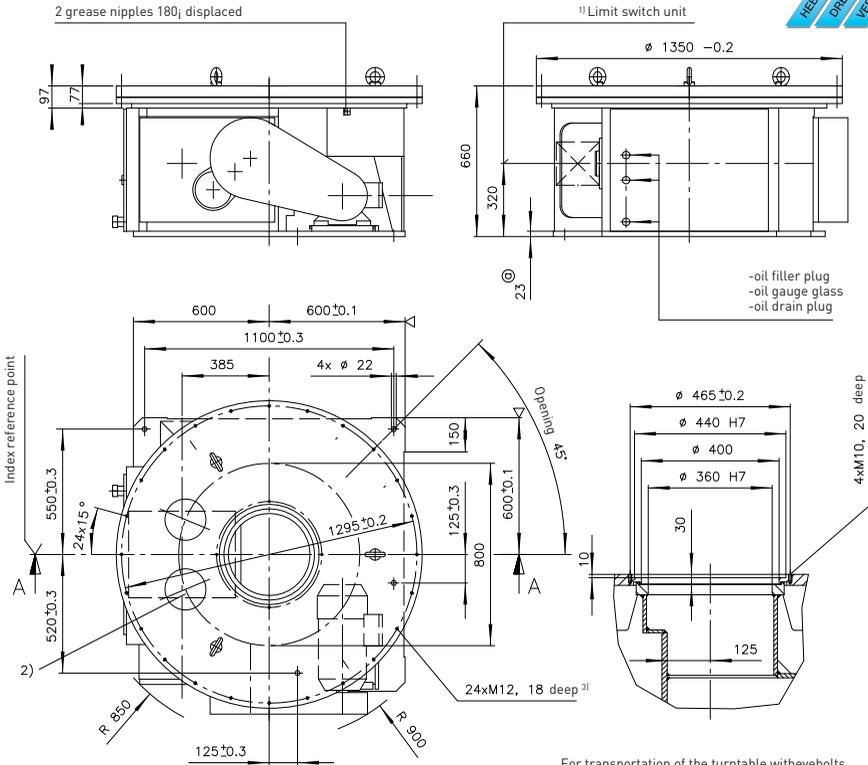
For transportation of the turntable with eyebolts, 3 tapped holes M24x40 deep have been arranged on  $\varnothing 935$ .
