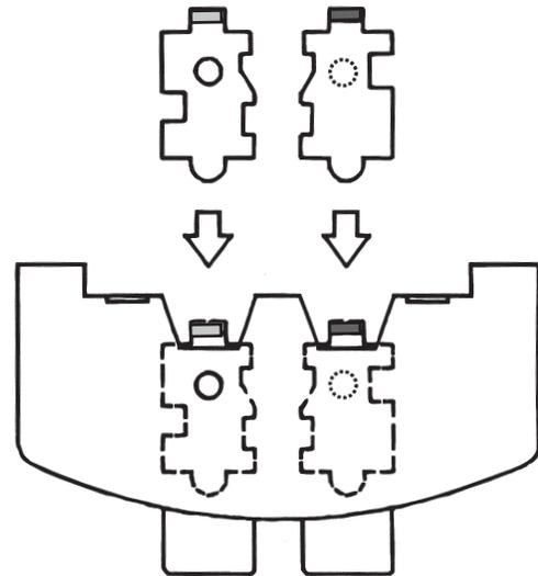
While holding knob in clear position make sure the blue or red colored end of the tumbler is facing upwards. Make sure notch is placed in the correct insert of the tumbler slot. See example.
