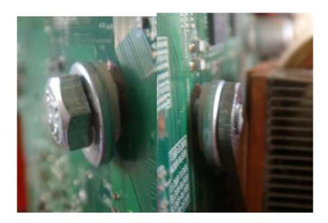
You need to attach both heat sinks to the motherboard. Above is a picture of the process. Put a metal washer first then a nylon washer and then insert the bolt into the mother board and now add another nylon washer and then another metal washer for all 4 holes. Now align the heat skink and bolts together and hand tighten the bolts to the motherboard, make sure no to over tighten the bolts.
