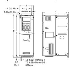
Dimensions are in millimeters and (inches).
