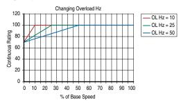
[Motor NP FLA] is multiplied by [Motor OL Factor] to select the rated current for the motor thermal overload. This can be used to raise or lower the level of current that will cause the motor thermal overload to trip. The effective overload factor is a combination of [Motor OL Hertz] and [Motor OL Factor].
