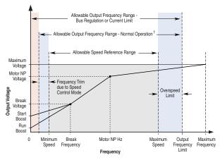
Note 1: The lower limit on this range can be 0 depending on the value of Speed Adder
