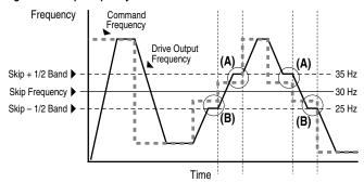
Some machinery may have a resonant operating frequency that must be avoided to minimize the risk of equipment damage. To assure that the motor cannot continuously operate at one or more of the points, skip frequencies are used. Parameters 084-086, ([Skip Frequency 1-3]) are available to set the frequencies to be avoided.
