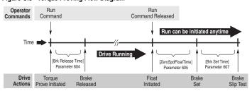
All times between Drive Actions are programmable and can be made very small (i.e. Brake Release Time can be 0.1 seconds)
