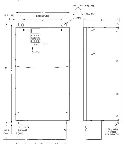
Dimensions are in millimeters and (inches)
