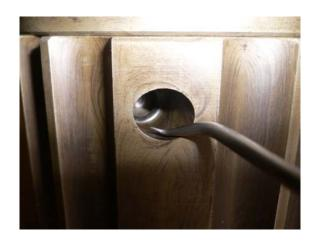
Push out the locking pins by inserting a suitable tool through the smaller holes in the pilot bit.
